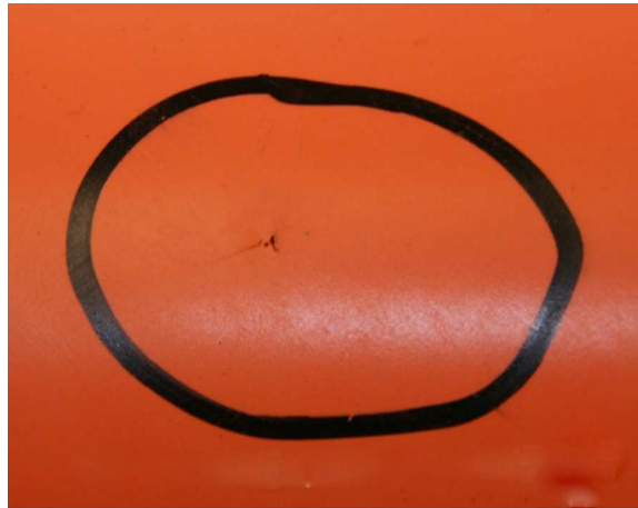
FIG. 5 Breakdown (Dielectric Failure Blanket: Front)
