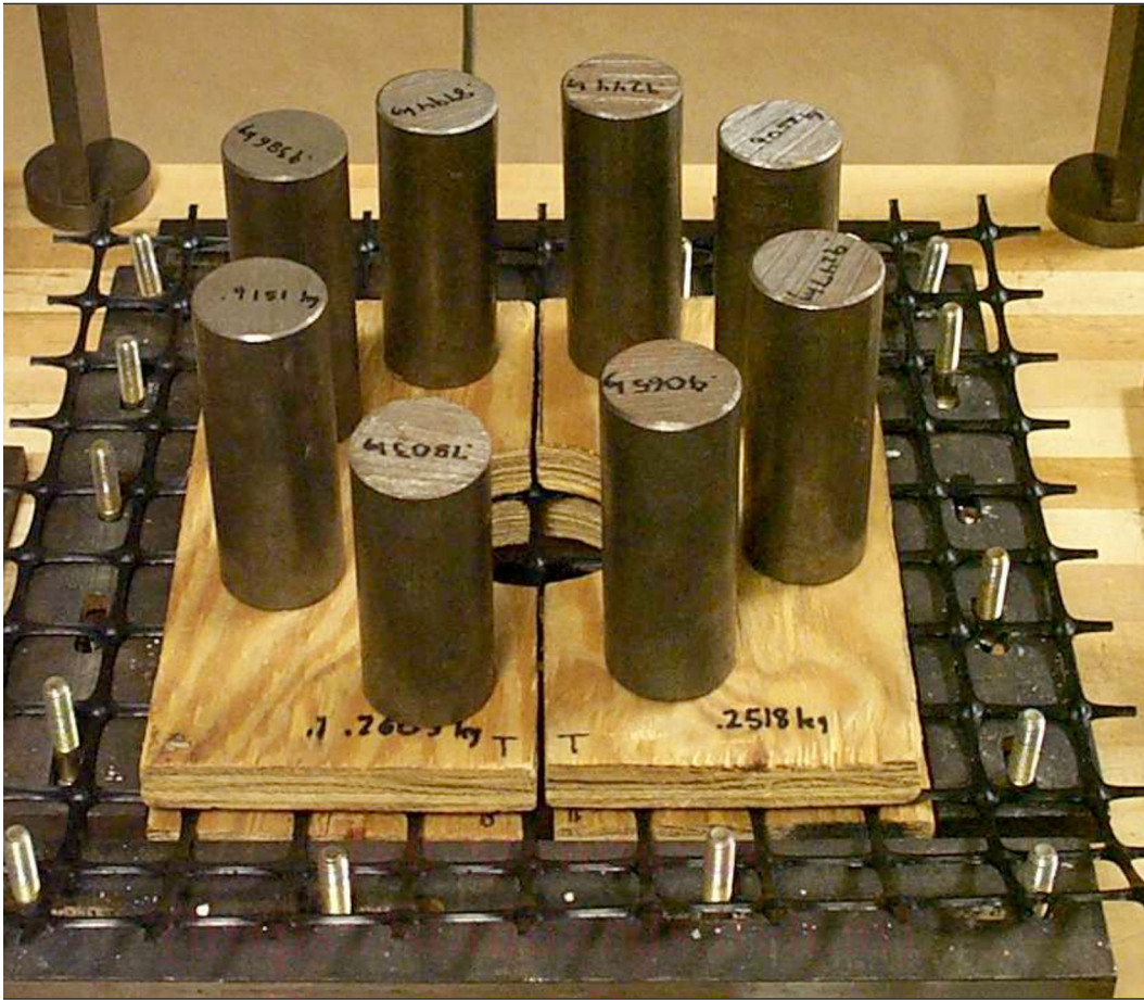
FIG. 3 Loading Plates and Weights Applied Prior to Clamping Specimens on Table Clamps
