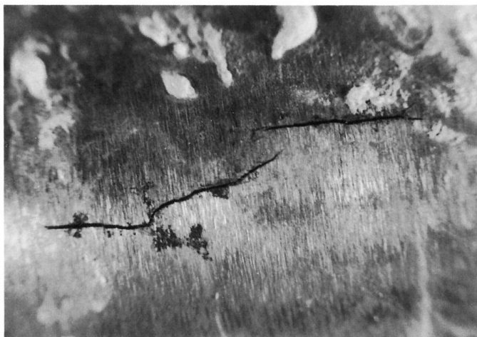
FIG. 2 Typical External Stress Corrosion Cracks (5× Magnification)
