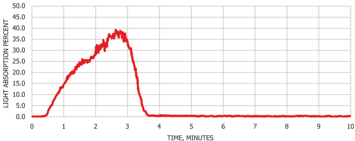
FIG. 10 Representative Time-Absorption Curve for Smoke Density of Heptane
