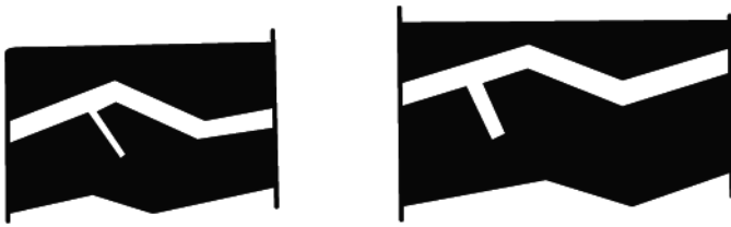
A SIPE WIDTH < 1 MM A NOTCH (CLOSED END) WIDTH > 1 MM FIG. 1 Schematic Diagrams Kerf (Sipe) and Notch
