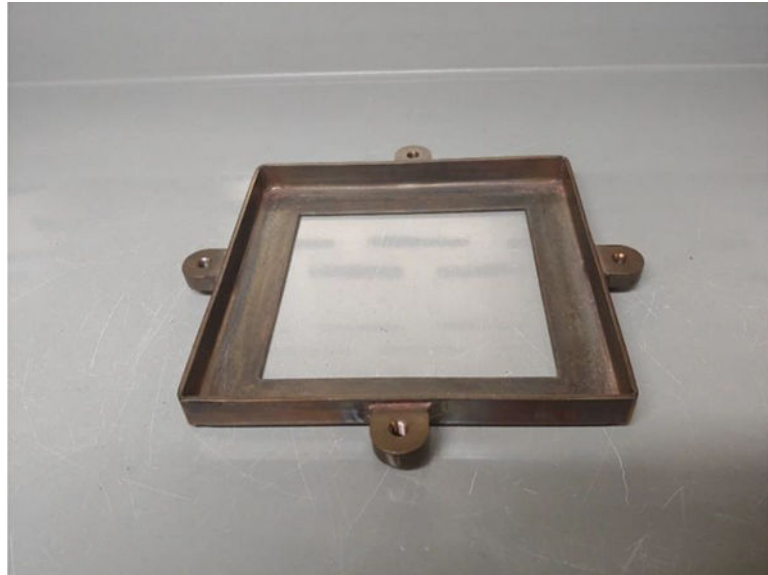
FIG. A1.1 Place the Top Retainer Frame Upside-down on the Bench
