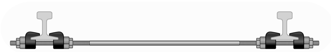
FIG. 1 Gauge Rods (installed on rails, ties and tie plates not shown)
