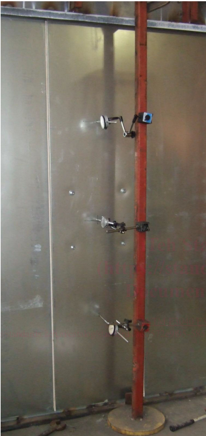
FIG. 1 Setup to Measure Deflection
