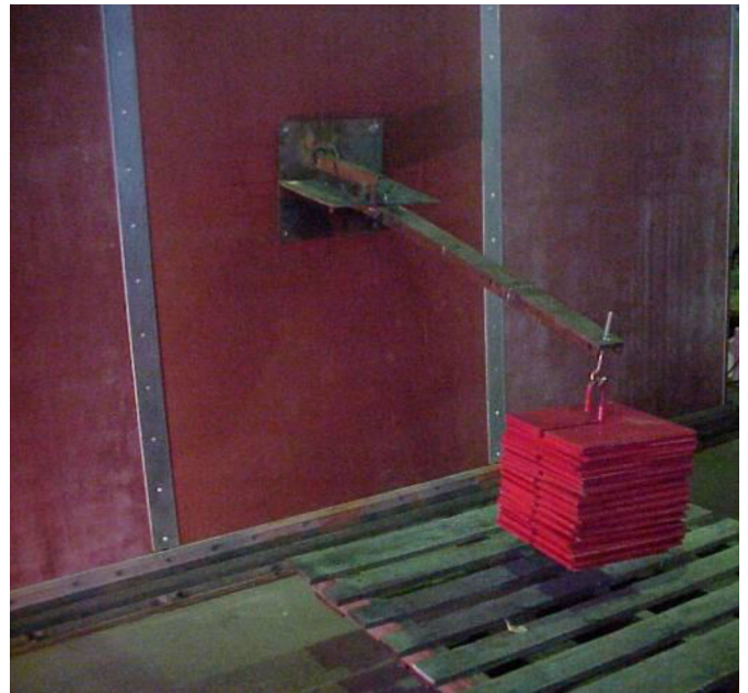
FIG. 2 Loading Bracket with Load Applied at 915 mm [36 in.]
