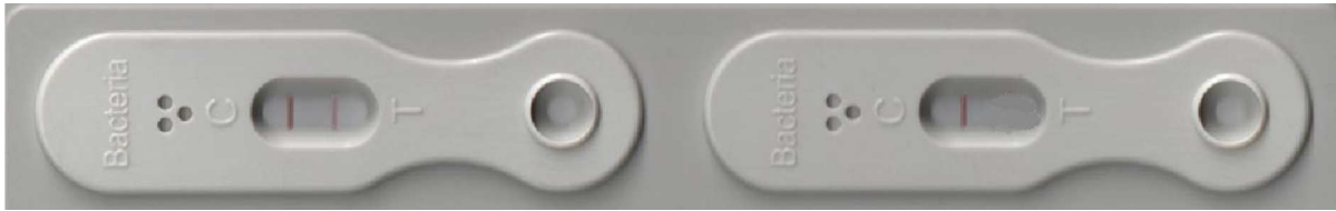
FIG. 4 Bacteria LFD Detecting >150 µg to ≤750 µg Antigen/L Fuel Phase or >33 µg Antigen/mL Aqueous Phase and ≤166 µg Antigen/mL Aqueous Phase: Test Lines are Visible Only on the High-Range (Left) LFD
