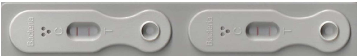
FIG. 3 Bacteria LFD Detecting \leq 150 \mu\text{g Antigen/L Fuel Phase} or \leq 33 \mu\text{g Antigen/mL Aqueous Phase} : Both Test and Control Lines Visible
