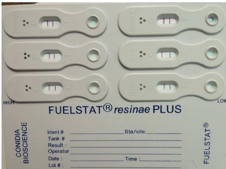
FIG. A1.1 LFD Tray Detecting \leq 150 \mu\text{g} Antigen/L Fuel Phase or \leq 33 \mu\text{g} Antigen/mL Aqueous Phase
