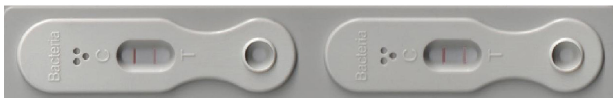
FIG. 3 Bacteria LFD Detecting ≤150 µg Antigen/L Fuel Phase or ≤33 µg Antigen/mL Aqueous Phase: Both Test and Control Lines Visible
