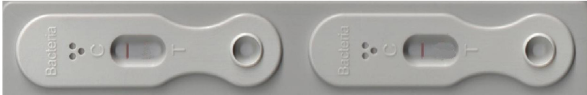
FIG. 5 Bacteria LFD Detecting >750 \mu\text{g} Antigen/L Fuel Phase or >166 \mu\text{g} Antigen/mL Aqueous Phase: No Test Lines Visible
