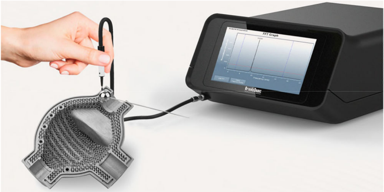
FIG. 6 Manual Operation of IEM System for AM Part Inspection
