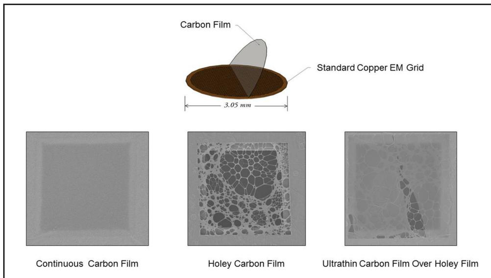
FIG. 2 The Three Different Types of Carbon Film on EM Grids That May be Used to Conduct Cryo-TEM of Liposomes
