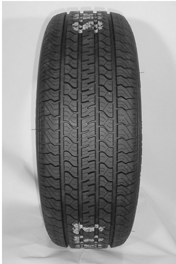
FIG. 1 Front View of the P225/60R16 97S Radial Standard Reference Test Tire
