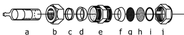
FIG. 2 Open-Face Filter Assembly: (a) Sampling Cartridge, (b) Inner Nut, (c) Back Ferrule, (d) Front Ferrule, (e) Union, (f) Front Ferrule, (g) Filter Support, (h) Filter, (i) Fluoroelastomeric or PTFE O-ring, (j) Outer Nut
