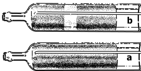
FIG. 1 PUF Sampling Cartridge (a) and PUF "Sandwich" Sampling Cartridge (b)
