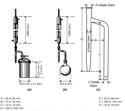
FIG. 1 Apparatus for Determining Water Content
