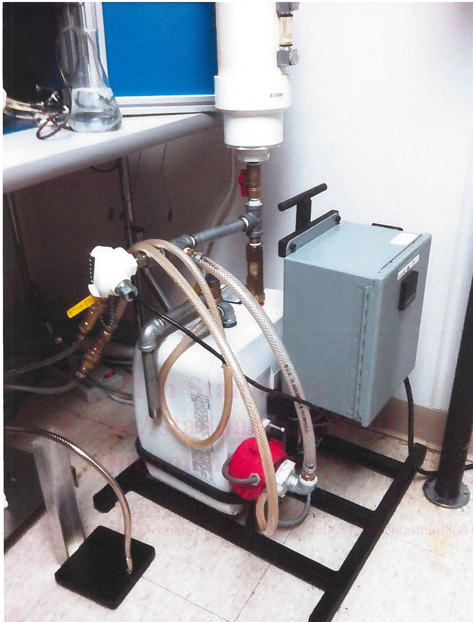
FIG. 3 Water Circulating System
