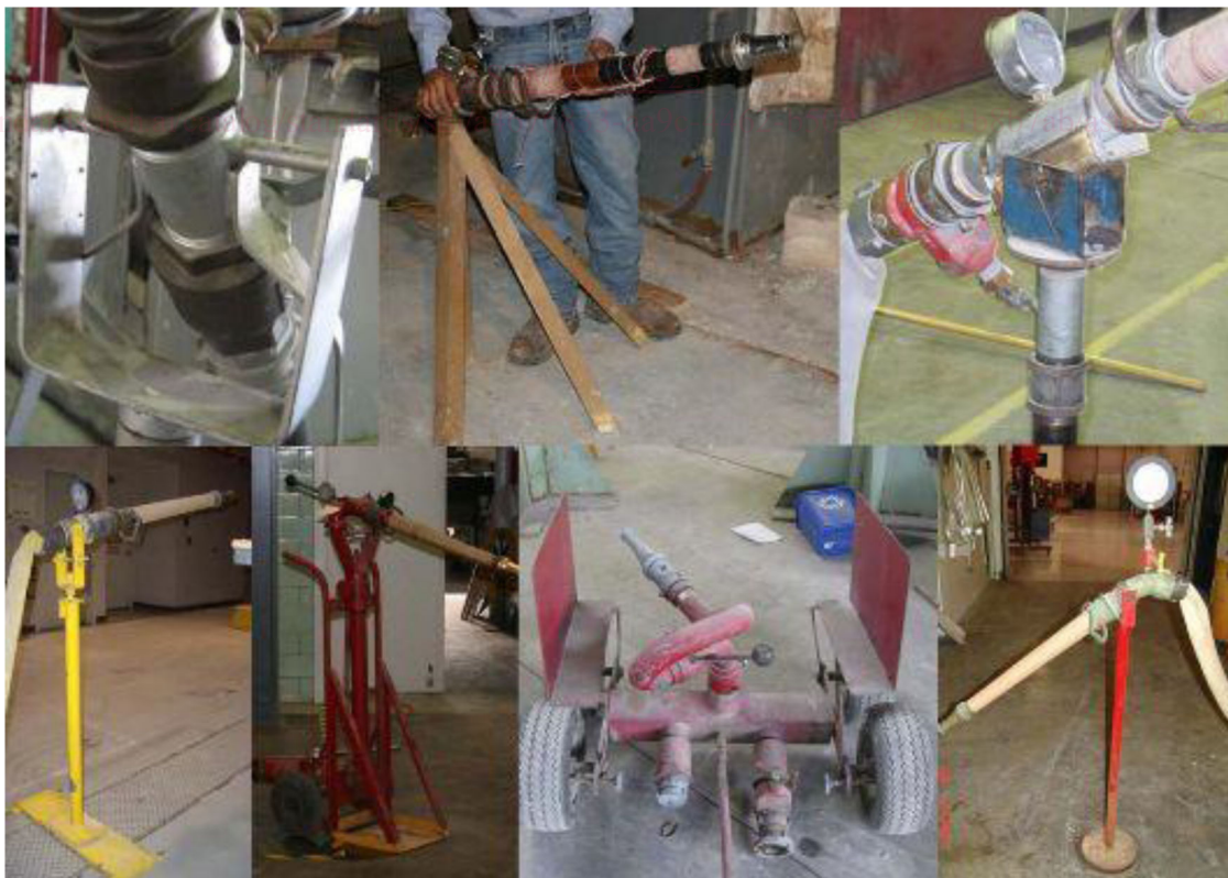
FIG. 2 Typical Hose Mounting Methods
