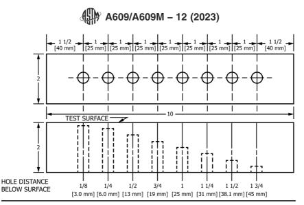
Note 1-Entrant surface shall be 250 µin. [6.3 µm] or finer.
