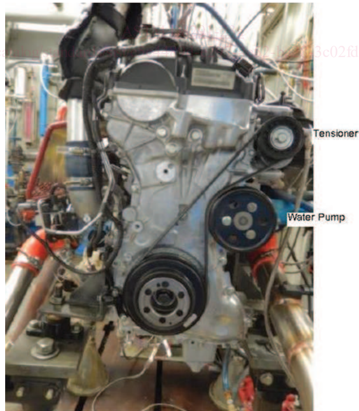
FIG. 3 Water-Pump Drive Arrangement
