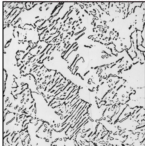
FIG. 1 Plate 1—IFI Spheroidization Rating
