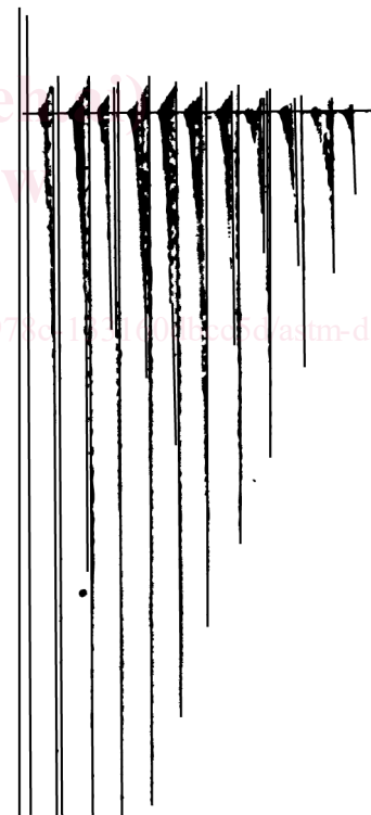
FIG. 12 Sample Drum Record of Impact Bending Test
