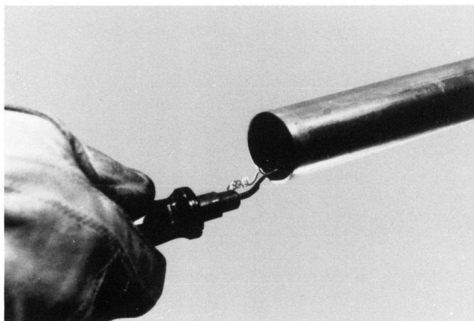
FIG. 5 Reaming: Deburring Tool
