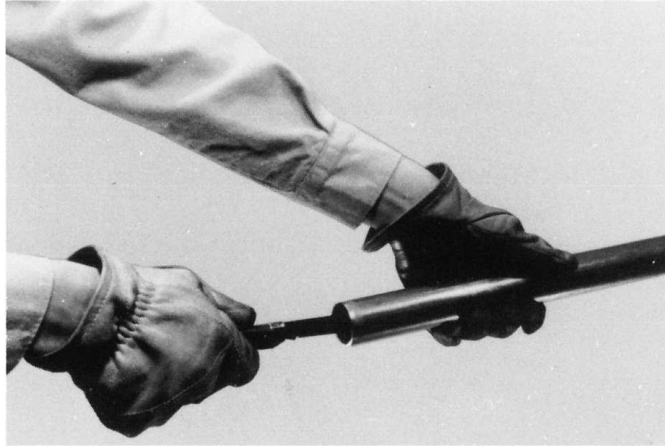
FIG. 4 Reaming: Pocket Knife
