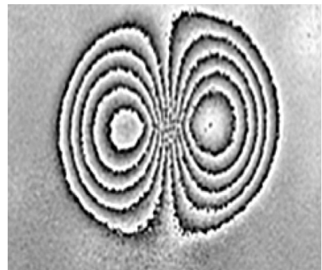
FIG. 4 A phase map shearogram with horizontal shear vector yields a fringe pattern showing the first derivative of the out-of-plane deformation, \partial w / \partial x . Using an unwrapping algorithm, the image at right shows the positive (white) and negative (black) slope change.
