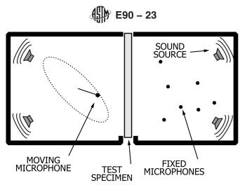
Note 1—This figure is not meant to be a design guide but is for illustrative purposes only. As an example, the room on the right has fixed microphones to measure average sound pressure level; the room on the left has a continuously moving microphone to measure average sound pressure level. Usually both rooms will have the same microphone system. The loudspeakers in the rooms generate the incident sound fields for the measurement of level differences or sound decay rates.
