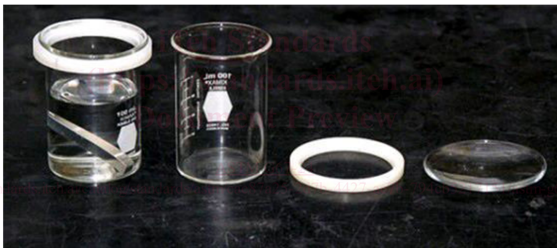
FIG. 1 Recommended Configuration for Specimen Exposure; A 100 mL Non-fluted Beaker and Watchglass
