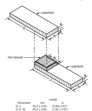
FIG. 1 Assembly of Test Sealant on Substrates
