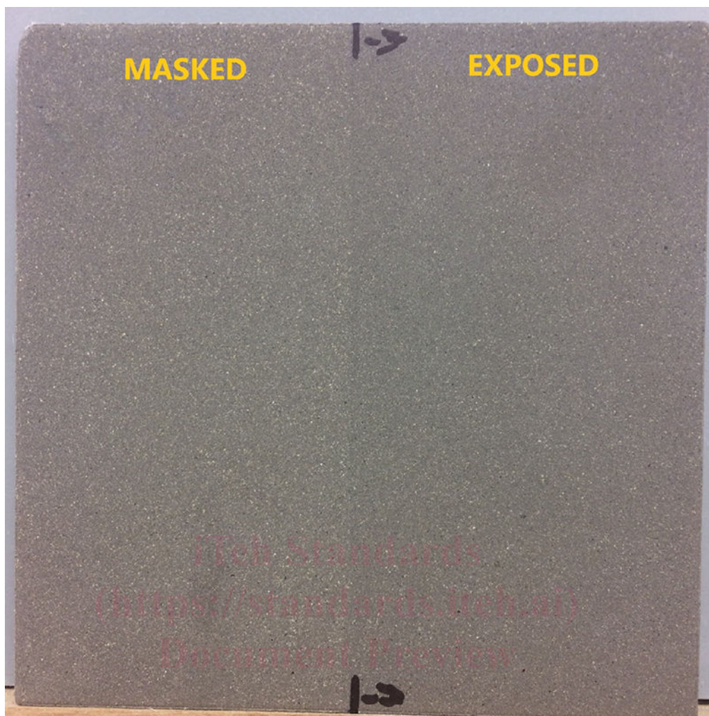
FIG. 1 Tile That Has Retained Grout After Testing
