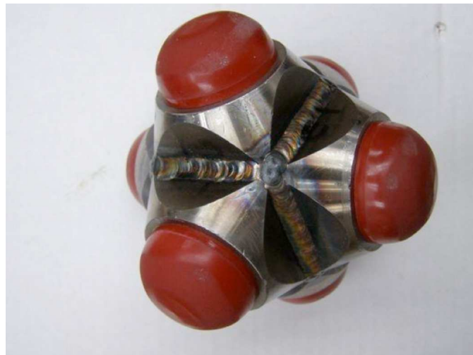
FIG. 3 8.4 lb Commercial Hexapod Tumbler
