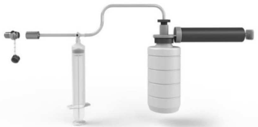
FIG. 2 Example of a Dissolved Gas Device
