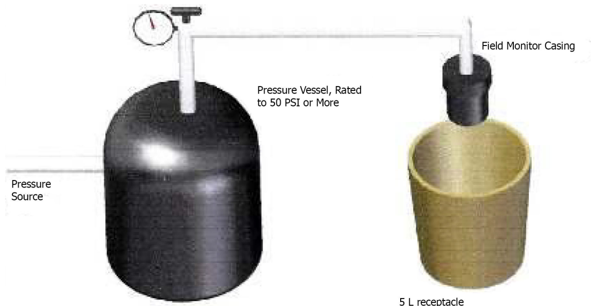
FIG. 1 Test Apparatus for Seal Assessment: All Components to be Electrically Bonded Together and Grounded
