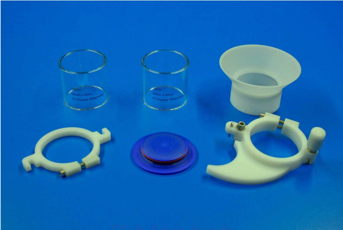
FIG. 4 Components Required to Assemble the 50-mm x 85-mL Shear Cell Vessel (4-mm ball-ended hex key not shown)
