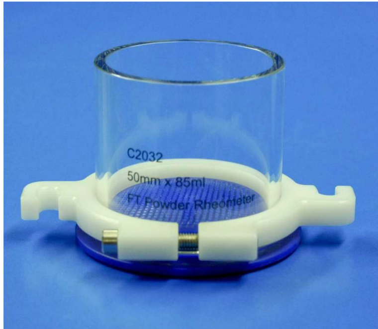
FIG. 6 Fitting the Serrated Base with O-ring to the Glass Cylinder
