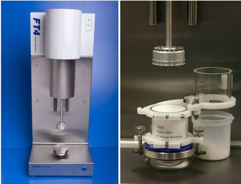
FIG. 1 FT4 Powder Rheometer (The left hand image shows the instrument with the shear head fitted; the right hand image shows the shear head and shear cell test vessel.)
