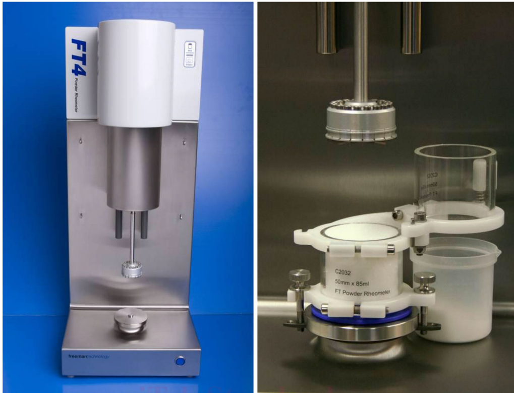
FIG. 1 FT4 Powder Rheometer (The left hand image shows the instrument with the shear head fitted; the right hand image shows the shear head and test vessel.)
