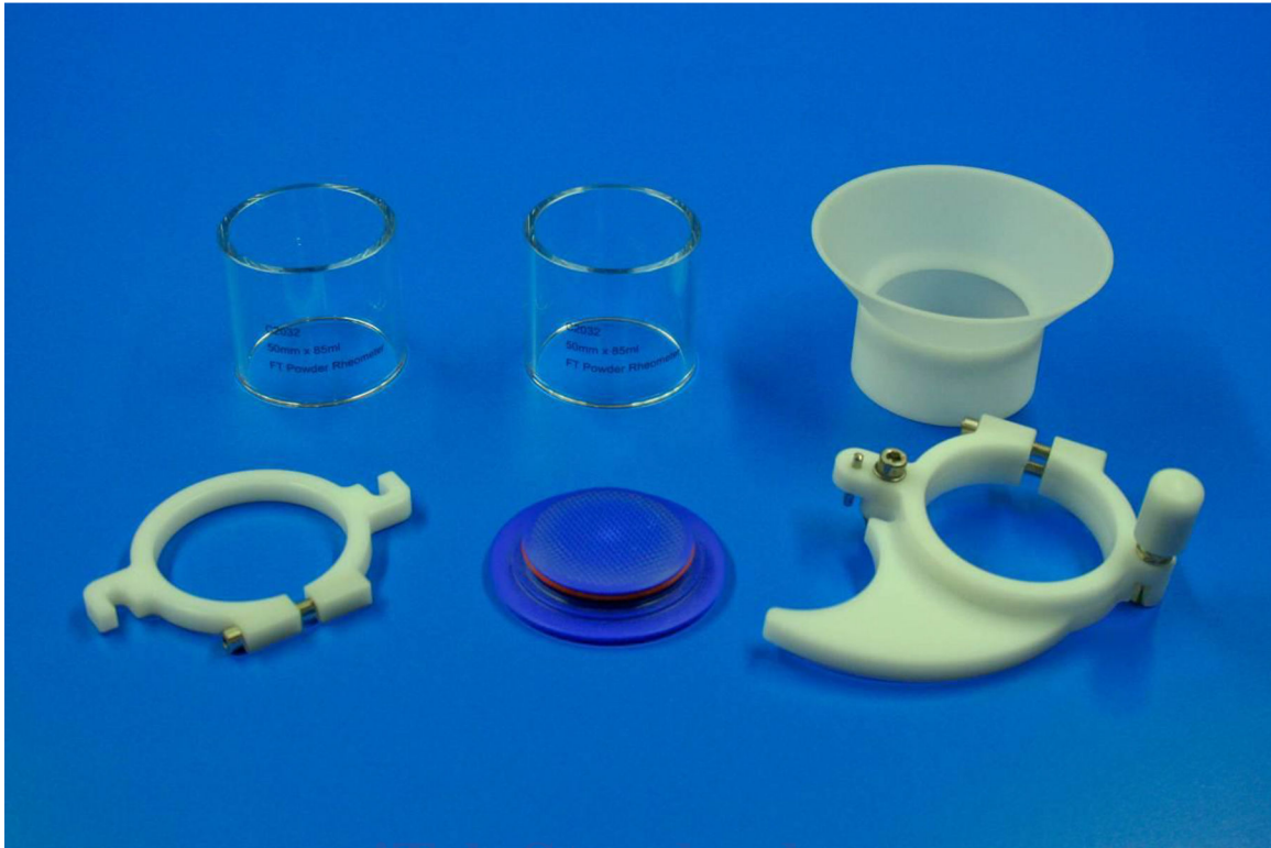
FIG. 4 Components to Assemble the Shear Cell Vessel (4-mm ball-ended hex key not shown)
