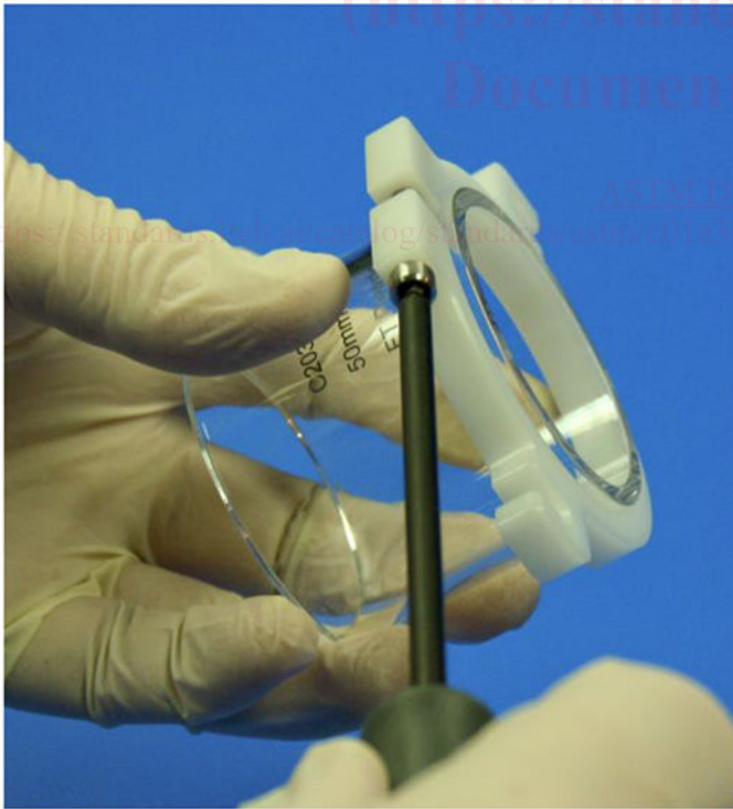
FIG. 5 Fitting the Clamp Ring to the Glass Cylinder Using the Ball-ended Hex Key
