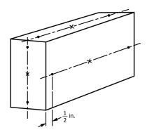
Note 1—The dots on the center line of each face are  $\frac{1}{2}$  in. (13 mm) in from each edge, and the cross on the axis is in the center. These positions indicate the points at which three measurements for each dimensions are to be made.
