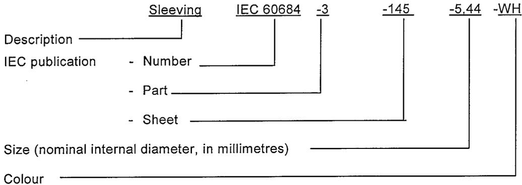
Any abbreviation used for colour shall comply with IEC 60757 where applicable. The abbreviation for non-coloured shall be "NC". Non-standard colours shall be written out in full.
