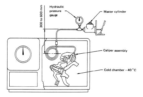
Figure 2 — Low temperature leakage test
