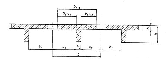
Figure 2.102: Definitions of dimensions of effective width of flanges
