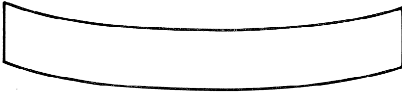
Unacceptable deformation (Centre lower than the ends)
