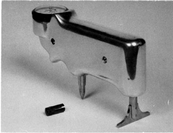
FIG. 1 Barcol Impressor, Model 934-1
