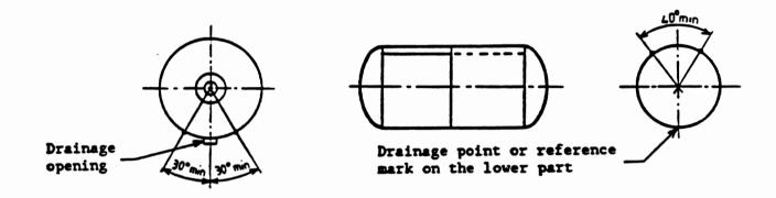
Figure 1: Position of longitudinal welds on the bottom of the shell
