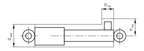
Figure 3 — Cross sectional dimensions of damper ( $D_{\rm max}, D_{\rm res}, H_{\rm res}$ )
