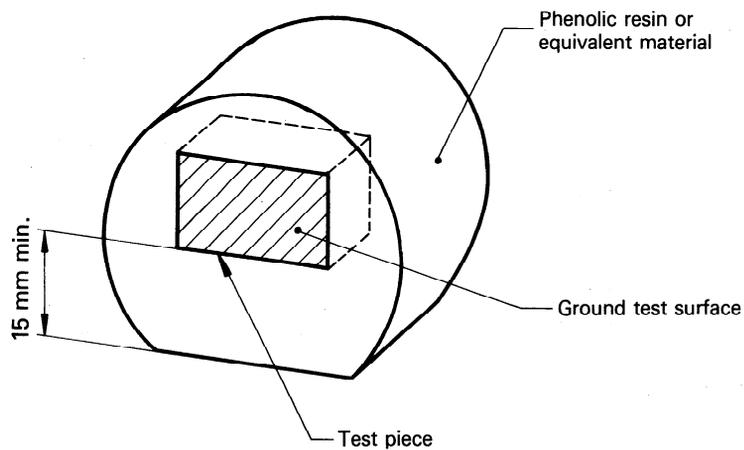
Figure 2 – Embedded test piece with one test surface
