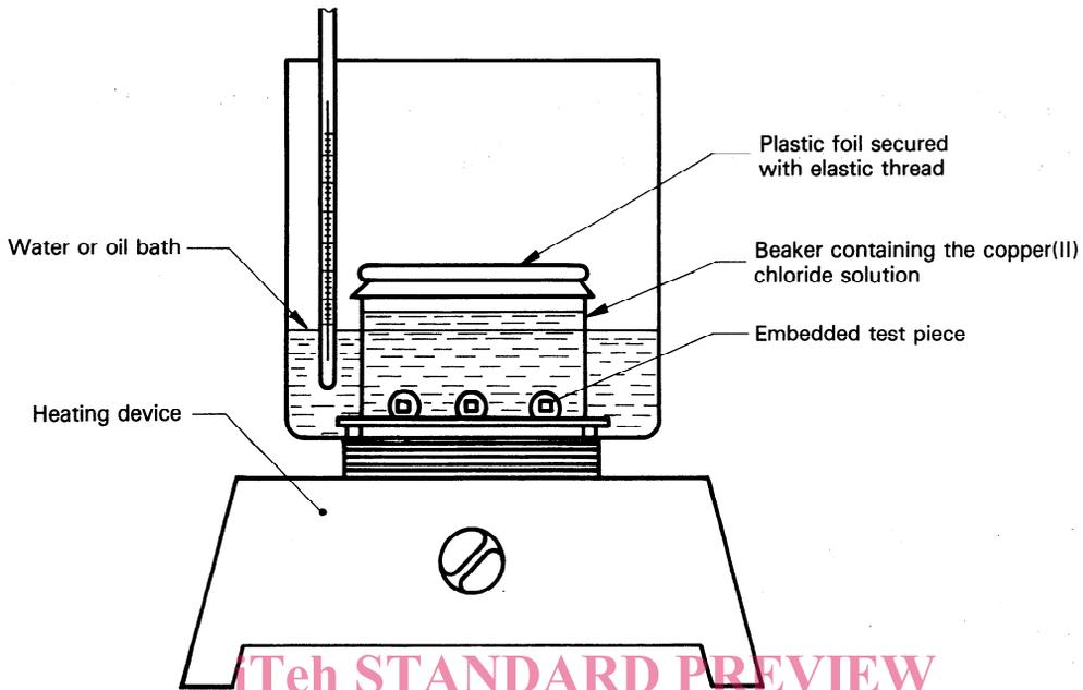
Figure 1 – Example of test apparatus
