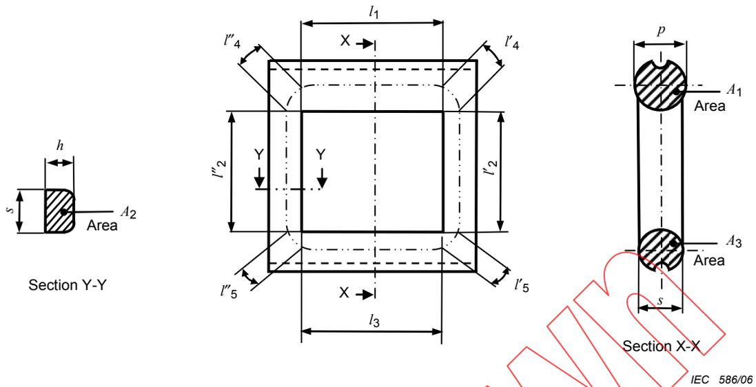
In calculating  $A_2$  ignore any ridges introduced for the purpose of facilitating manufacture.
