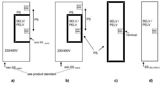
SS = Simple Separation = Basic Insulation for rated insulation voltage
