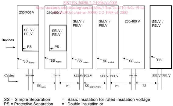
Figure 3 - Protective separation for adjacently mounted HBES devices
