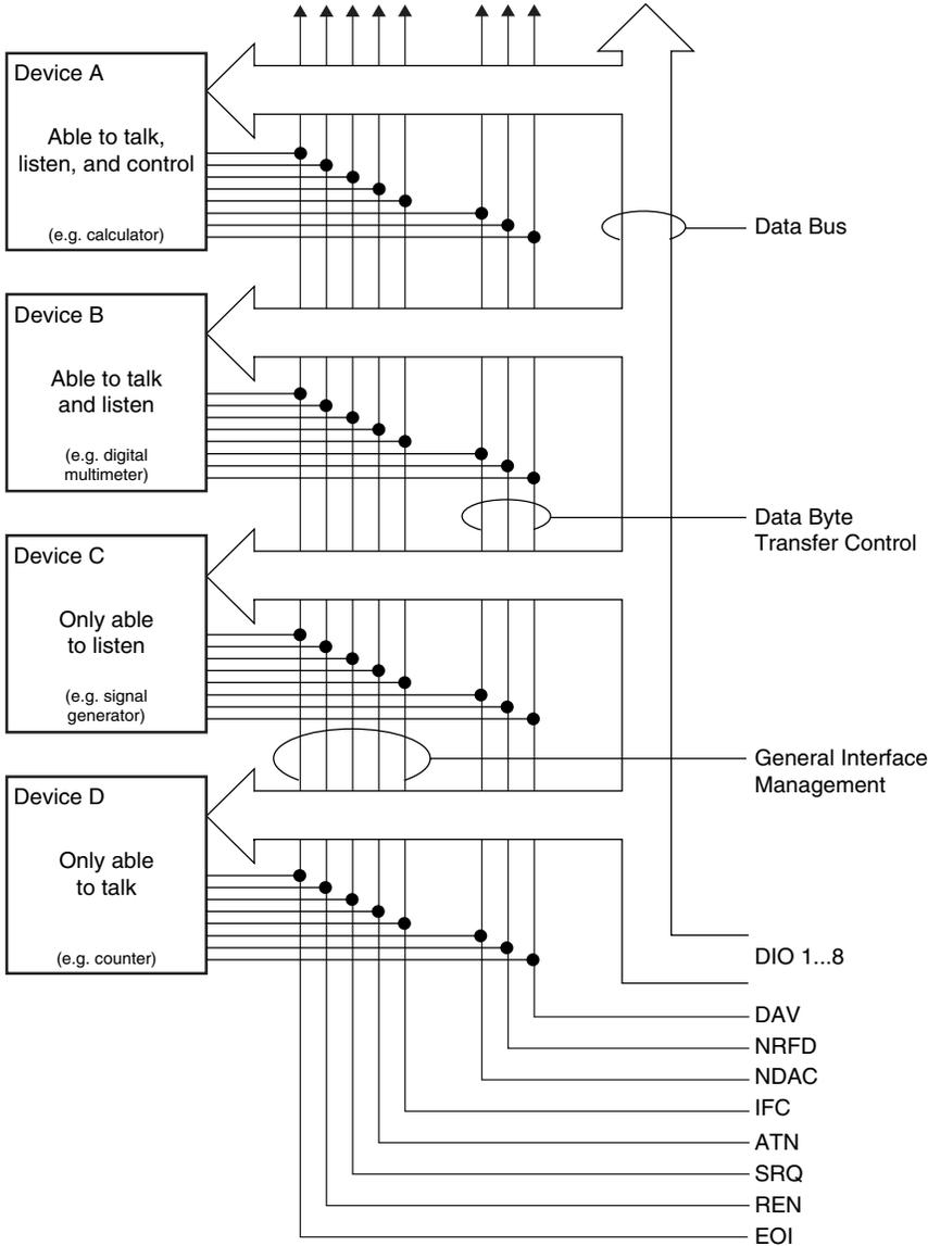
Figure 1—Interface capabilities and bus structure
