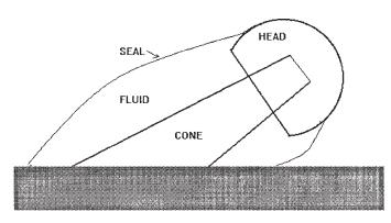
Note 1—For Method I, the fluid is contained within the sleeve. For Method II, the device should be submerged in an electrolyte while the contact area between the top of the head and the loading apparatus is not exposed to the fluid. A counter electrode is placed in the same bath.
