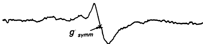
Figure A.1: Typical ESR spectrum of an unirradiated chicken thigh sample
