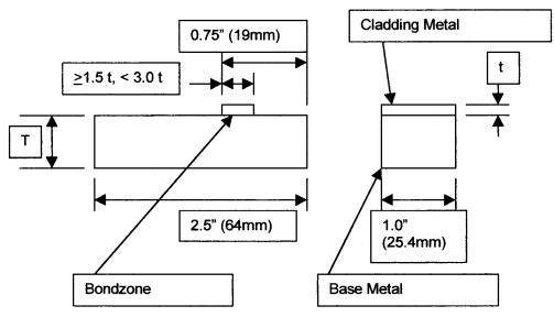
t = Cladding Metal Thickness—If > 0.125 in. (3.2 mm), machine to 0.125 in. (3.2 mm) max
