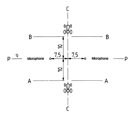
1) One microphone position may be eliminated, in which case an additional test run from BB to AA is required
