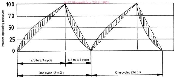
The curve shown above is the approximate pressure/time cycle for proper severity for surge testing hose assemblies. It is mandatory that the pressure peak rises to 100 % of nominal pressure. It is considered desirable that the pressure time curve be confined to the shaded area so that results of tests performed on different test machines will be more nearly comparable.
